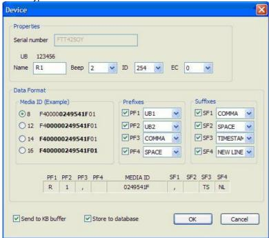
**Device/Edit pane** – used to set formatting and other parameters for a specific SL-287. The parameters are stored in the reader itself and are automatically used when the reader is attached to another PC.
