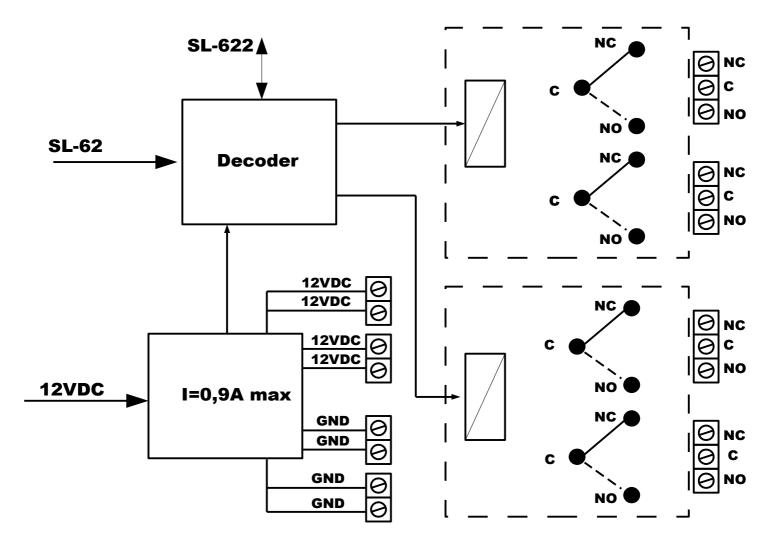
The above block diagram shows the elements of the SL-621 relay module.
