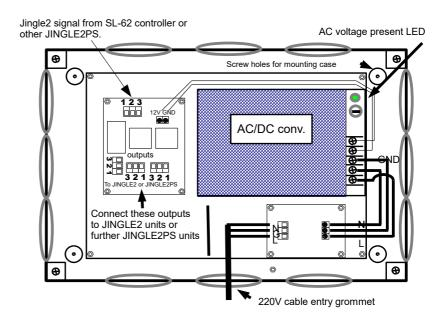
As the above drawing shows, the JINGLE2PS unit is housed in a 25x19.5cm plastic case with rubble cable glands on all sides. It contains the following elements:
