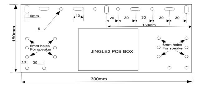
It has several round and elliptical mounting holes along the top and bottom sides and can be mounted onto cable-duct supporting struts which can usually be found going round factory production halls.
