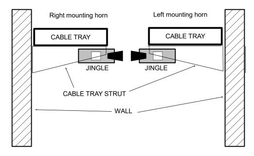
With this type of mounting, the carrier plate is pointing in the direction of the shop floor, i.e.. the direction of the horn-speaker. If the plate must be mounted parallel to a wall, the horn should be mounted onto the plate pointing inwards (towards the PCB box) because it can then be rotated
